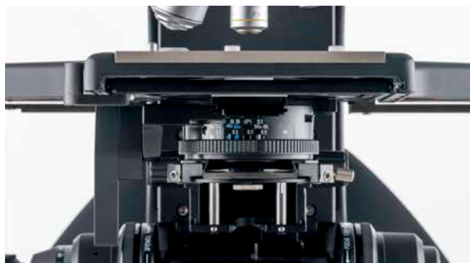
The aperture diaphragm's scale on the condenser has color markings matching the objective color codes.
